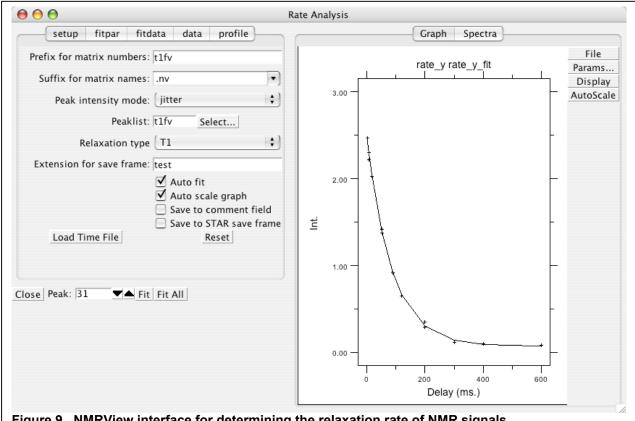
Figure 9. NMRView interface for determining the relaxation rate of NMR signals.
