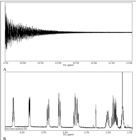
Fig 2. NMRView spectrum widget showing time domain and frequency domain signals.
